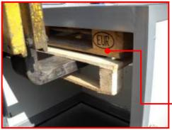
By removing the front door, it is possible to lift the structure by placing the forks of a forklift on the
