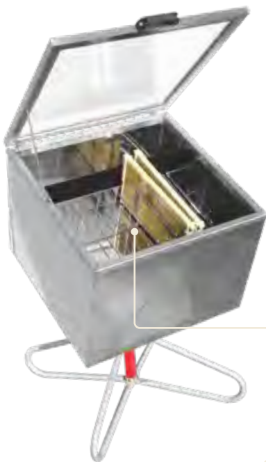
7150HS SOLAR WAX MELTER "SOLARE SOLARIS" with increased height in stainless steel sheet which allows the confining of the frames in a standing position inside the wire support. The wax immediately flows into the bowl, not soaking the esuvia that remains dry on the frame - 700x700 mm.
